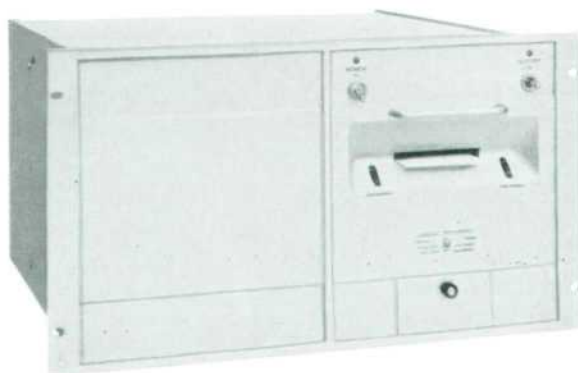
Fig. 1. -hp- Model 561A printer provides fast print-outs for digital data devices such as digital voltmeters, analog-digital converters, etc., that provide an output in 10-wire code form. Print-outs can be made of 11 columns at rates up to 5 lines per second.
